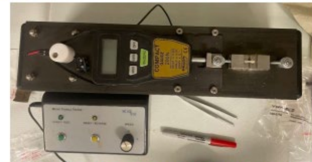
Figure 3. Micro-tensile strength of the specimens was tested with Microtensile tester.
