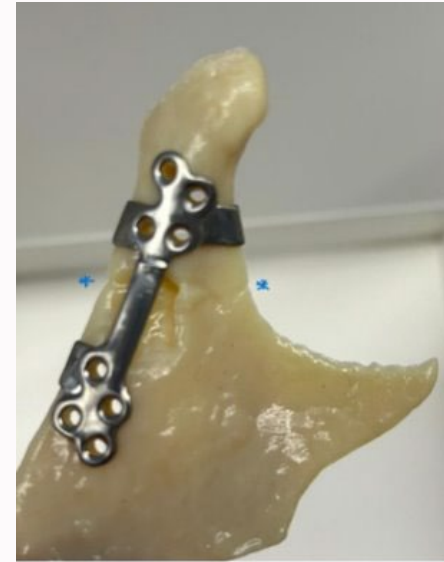
Sample of patient-specific implant with rigid plate construction, small tabs / hooks to assist in placement on bony edges and small indentation to assist in placement along fracture line.
